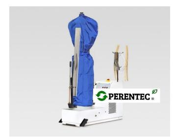
Ideal unit for the finishing of coats, jackets, dresses etc. The working cycles are completely automated thanks to an electronic card with which it is possible to set nine different cycles and to regulate the steaming and the drying time.
